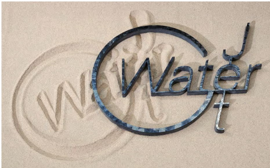
Water jet logo on 4 mm thick carbon fiber
