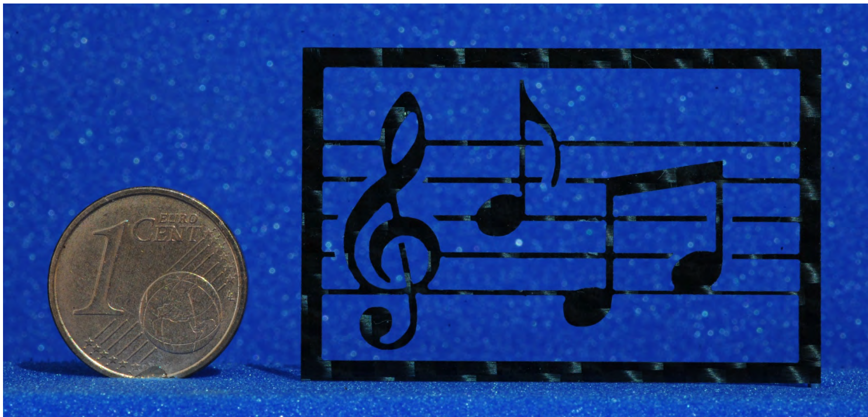
Musical notes and thin walls on 0.4 mm thick carbon fiber plate
