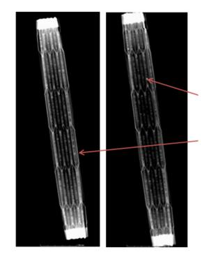
The experiment revealed interesting features that HALDOR-TOPSØE had not considered before seeing the results of neutron imaging. The arrows indicate the inhomogeneities identified within the stack.
