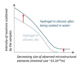
Fig3. Analysis of scattered intensity showing absorbing properties and hydrogel structure
