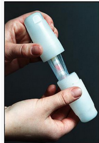
Fig. 2 Encapsulation of the sample before final packaging in an irradiation container. The container is then sent to a position close to the reactor's core by means of a pneumatic tube system.
