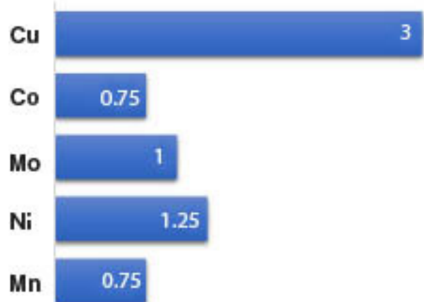
Fig. 3 Total Uncertainty of Neutron Activation Analysis for concentration measurements in A4-grade stainless steel, [1 standard deviation in %].
