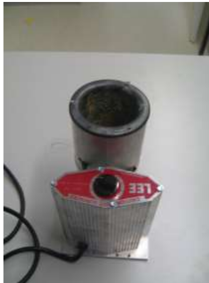
Oven – especially made for small lead spheres (old guns)
